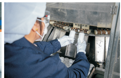
Electrical End Test Capacitance, dissipation, impedance test.
