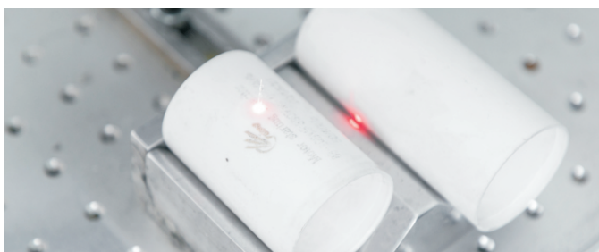
Label Printing Printing rating labels on capacitors.
