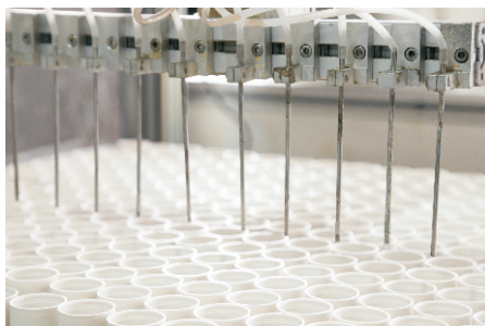
Coating Lacquering Filling insulating fluid for protection.
