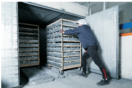
Heating and Drying 1 hour in 80°C, 7 hours in 95-100°C
