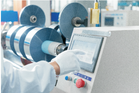
Film Slitting Slitting the metalized mother rolls.
