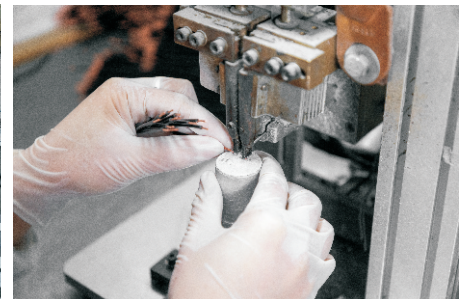
Terminal Welding Welding terminals on the end contract
