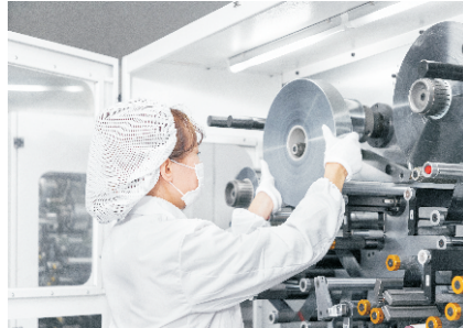
Winding High-Speed winding metalized film.
